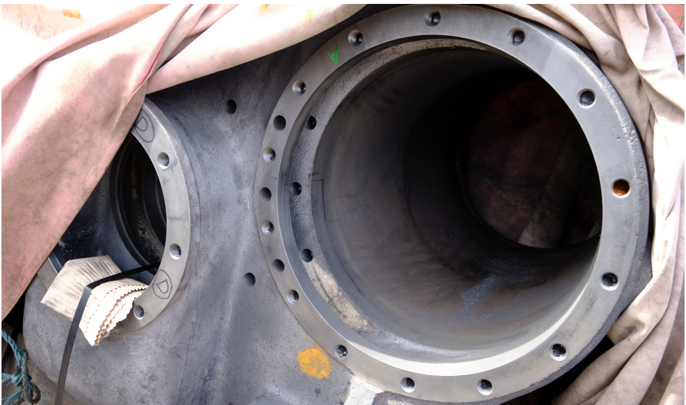
One of 4709's newly cast and machined cylinders spotted at Tyseley this week
