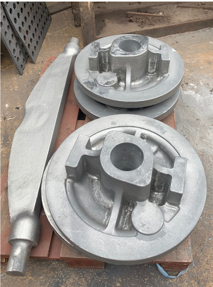
Fresh from the foundry, awaiting machining
