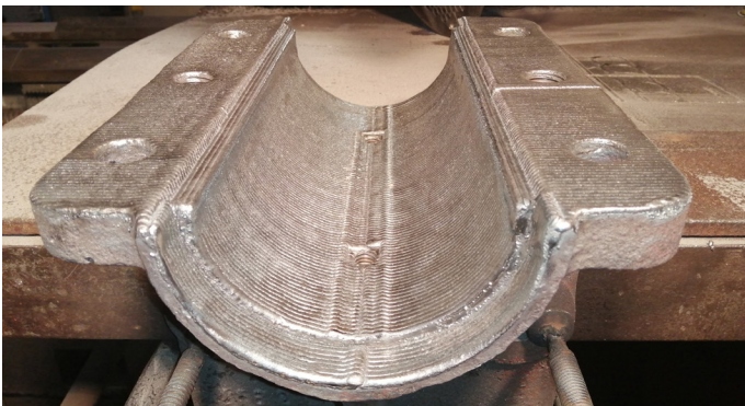
Above; Rockshaft bracket top after laser welding.
